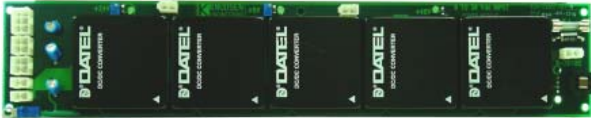
Figure 8.6: Power Distribution Module
